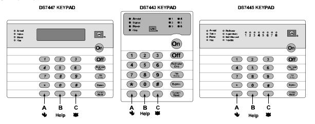
The Emergency Alarm Keys [A], [B], and [C] may generate Fire, Special Emergency, and Panic Alarms if programmed by the installer. Ask your installing company to explain the function of these keys.
